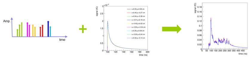
To be more realistic, effects from the electronic noise and electronic response can be introduced to the waveform
