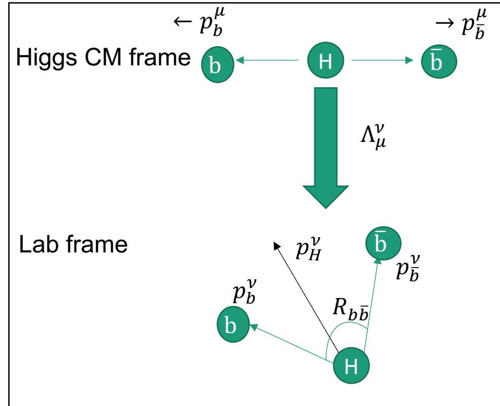
$$p_H^\nu = \left( p_H^0, \vec{p}_T^H \right) \quad |\vec{p}_b| = z |\vec{p}_T^H|, \quad |\vec{p}_{\bar{b}}| = \bar{z} |\vec{p}_T^H|$$
