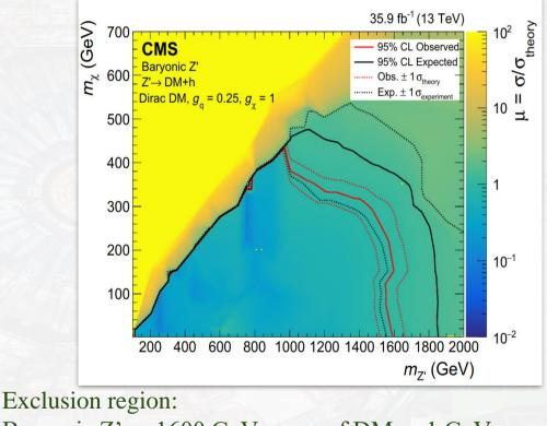
Baryonic Z': ~ 1600 GeV, mass of DM: ~ 1 GeV ~ 960 GeV, mass of DM: ~ 430 GeV
