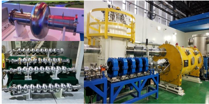
High Q SRF Cavity & Module
