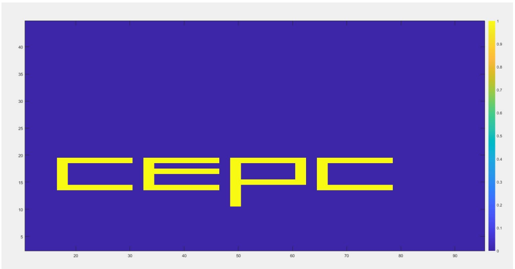
Fig.1 TaichuPix3 self-test with only several pixels turned on
