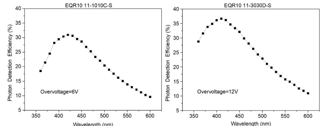
The PDE versus overvoltage and wavelength, deducted crosstalk and afterpulse and measured at 20 °C .
