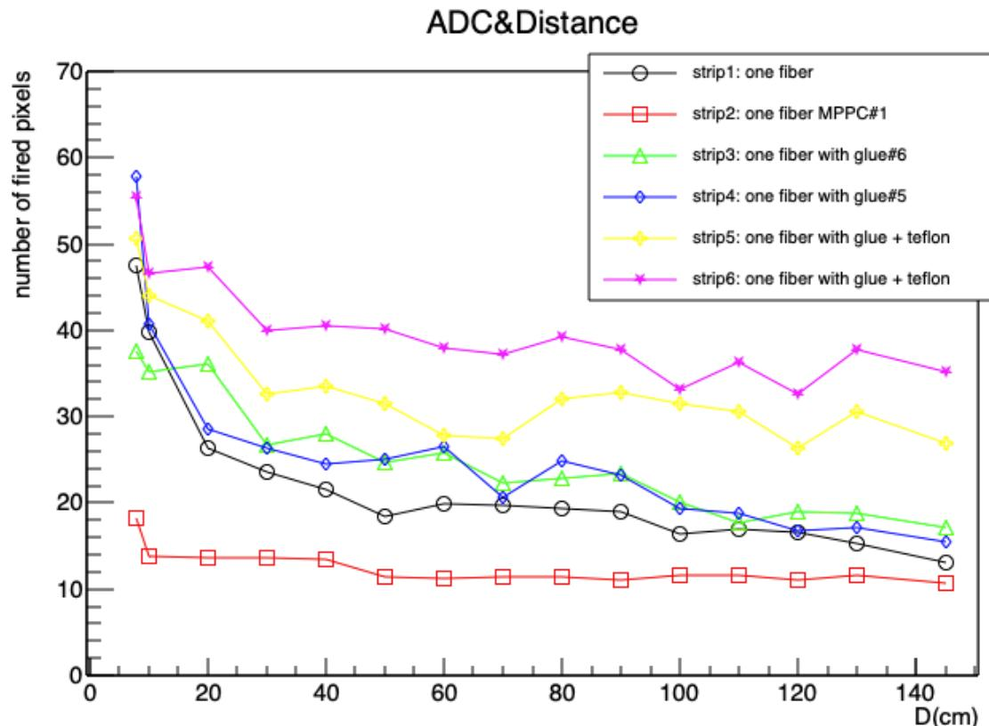
➤ Wavelength-shifting fiber keeps good photon collection at long distance
