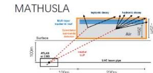
**Fig. 1:** Simplified detector layout showing the position of the  $200\text{ m} \times 200\text{ m} \times 20\text{ m}$  LLP decay volume used for physics studies. The tracking planes in the roof detect charged particles, allowing for the reconstruction of displaced vertices in the air-filled decay volume. The scintillator surrounding the volume provides vetoing capability against charged particles entering the detector.
