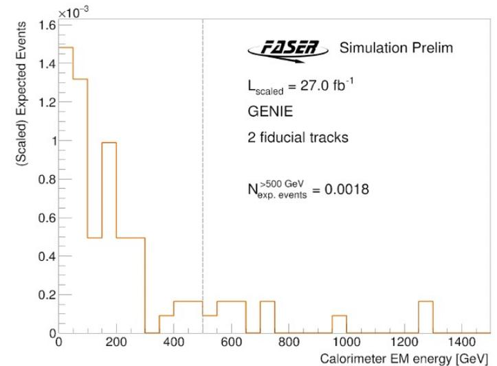
Non-collision background from cosmic and near-by beam debris is negligible. Studied in non-colliding bunches and runs without beam. No such events seen with  $E > 500 \text{ GeV}$  or a reconstructed track
