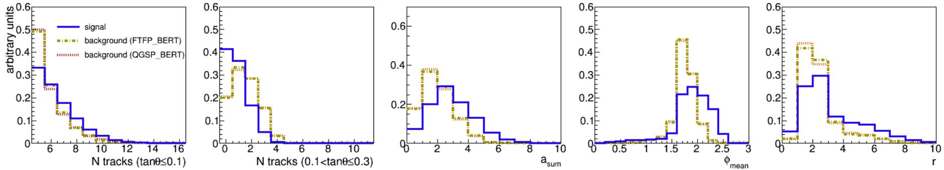
Five kinematic variables are used to separate signal and background
