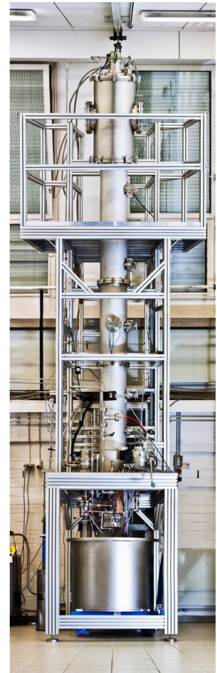
XENON1T/nT Kr distillation column
