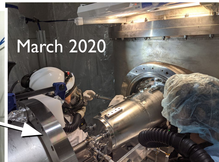
Making up cathode connections (under N2 purge)
