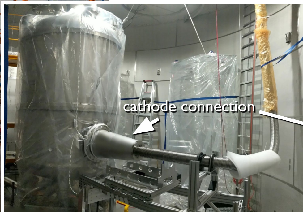
Making up cathode connections (under N2 purge)
