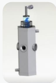
Thermo catalytic operando cell
