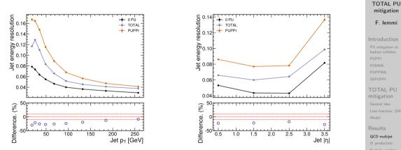
Jet energy resolution as a function of jet p<sub>T</sub> (left) and jet η (right)
