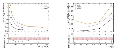
Jet energy resolution as a function of jet p<sub>T</sub> (left) and jet η (right)
