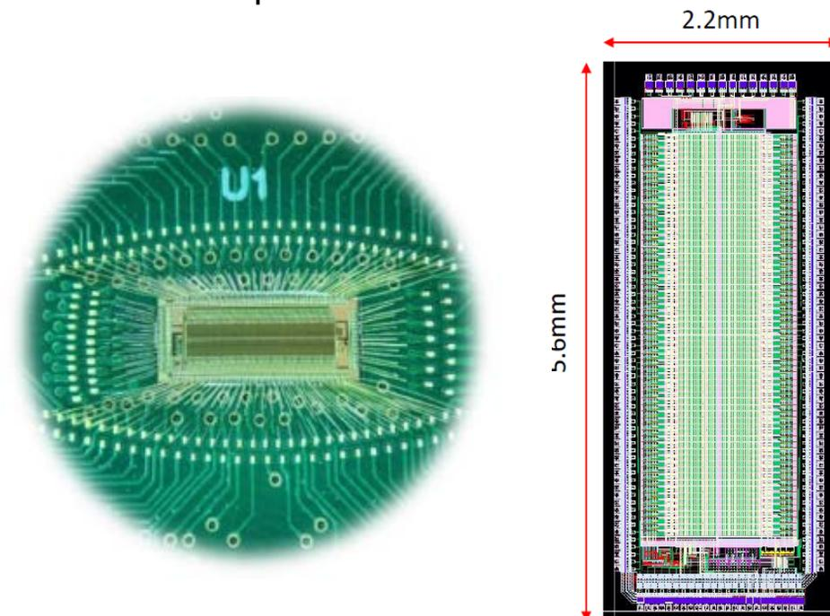
1<sup>st</sup> readout PCB board and the ASIC layout
