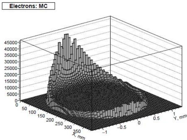
**Figure 4.** Recoil electrons at the detector. Number of  $x$ -bins is reduced to 100 for better visualization. Electrons detector covers the beam at the coordinates  $X = 0, Y = 0$ , which is impossible to do in practice.
