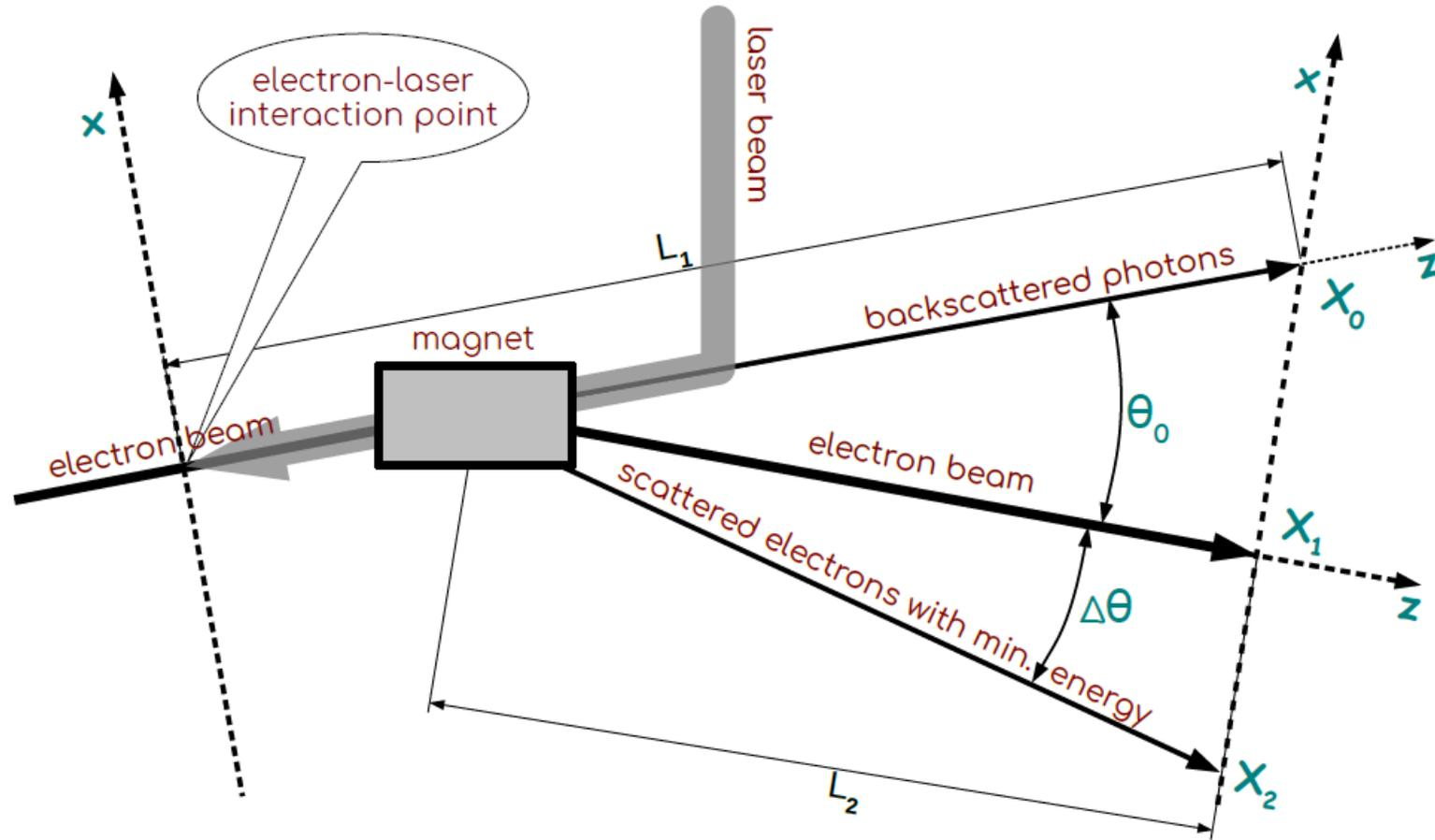
Figure 1. Layout of ICS experiment.
