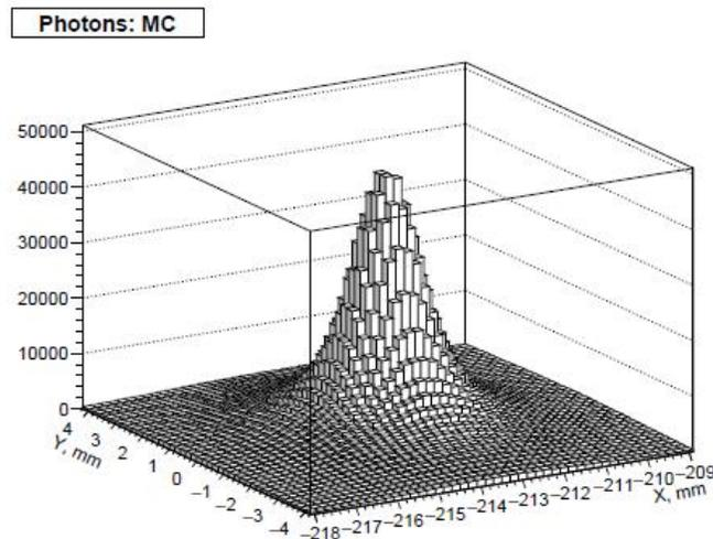
Figure 3. Photon spot at the detector. Number of bins is reduced for better visualization.
