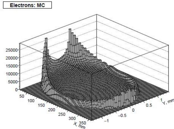
**Figure 5.** Recoil electrons at the detector. Number of  $x$ -bins is reduced to 100 for better visualization. Electrons detector is shifted in  $X$  by 15 mm away from the beam coordinates  $X = 0, Y = 0$ .
