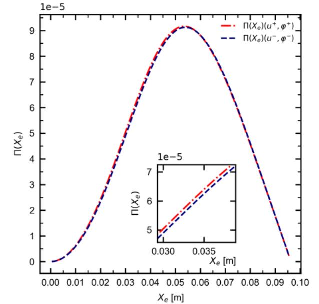
**Figure 5.** Graph of the analyzing power for CEPC Compton polarimeter. It is seen that in terms of the value of analyzing power, two sets of data denoted by blue and red curves are quite close and the maximum difference is merely  $10^{-6}$ .
