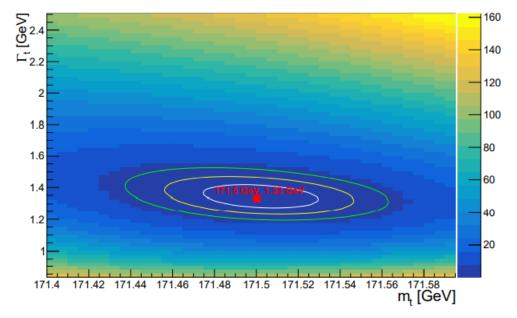
The uncertainty is 27 MeV on top mass and 72 MeV on width in the simultaneous fits of the two parameters using the energy points of 342.75 and 344.00 GeV.
