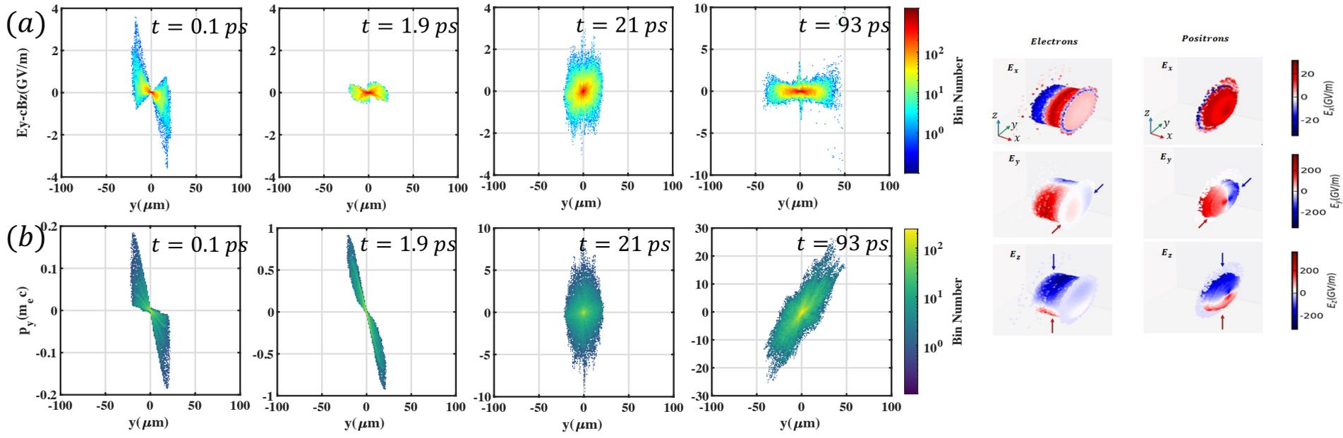
The transverse self-field of the relativistic driven electron beam can provide a transverse focusing force on the positron bunch. The process from focusing to short-term stabilization and finally weak defocusing until the transverse field is zero.
