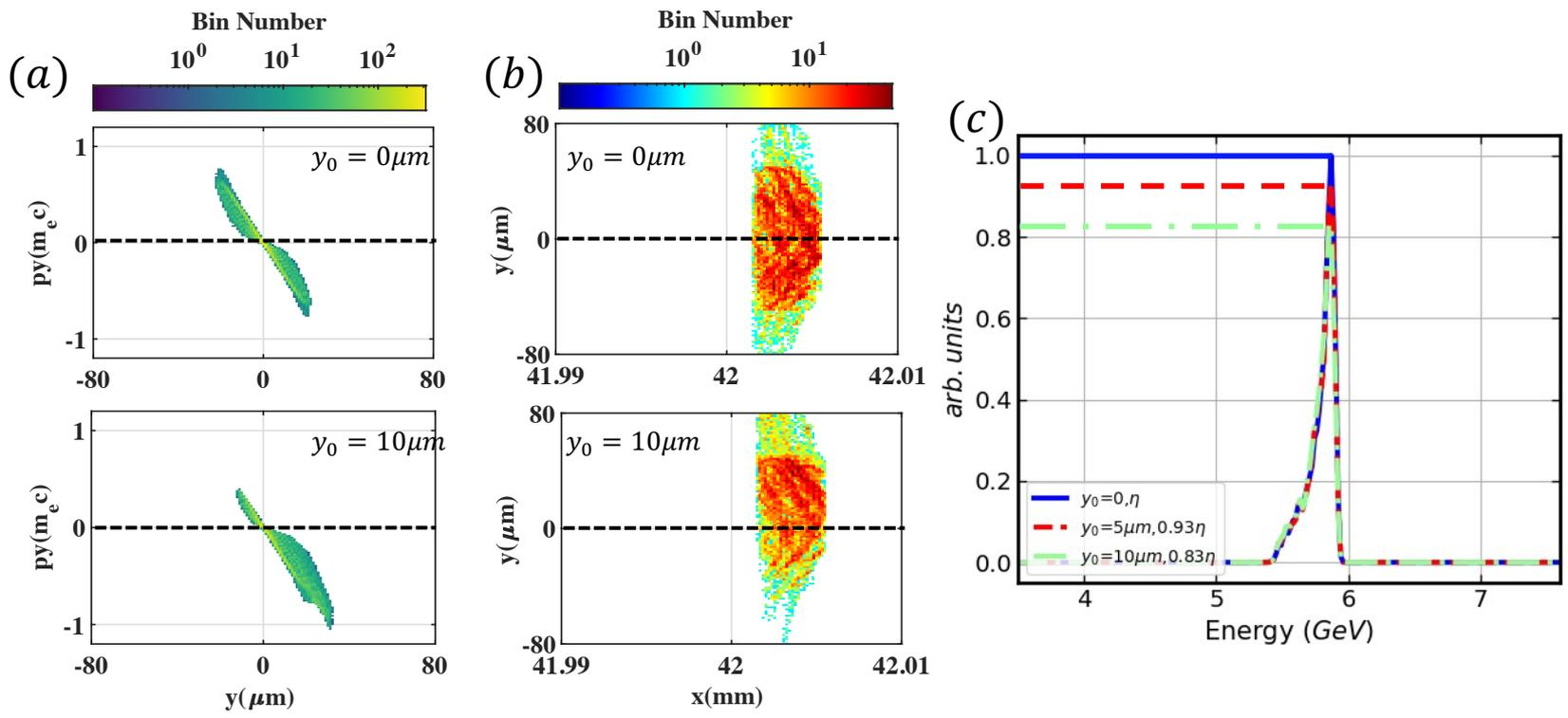
The energy transfer efficiency of positron bunch decreased by about 17% when the positron bunch deviated by 10  $\mu m$  transversely at the initial time.
