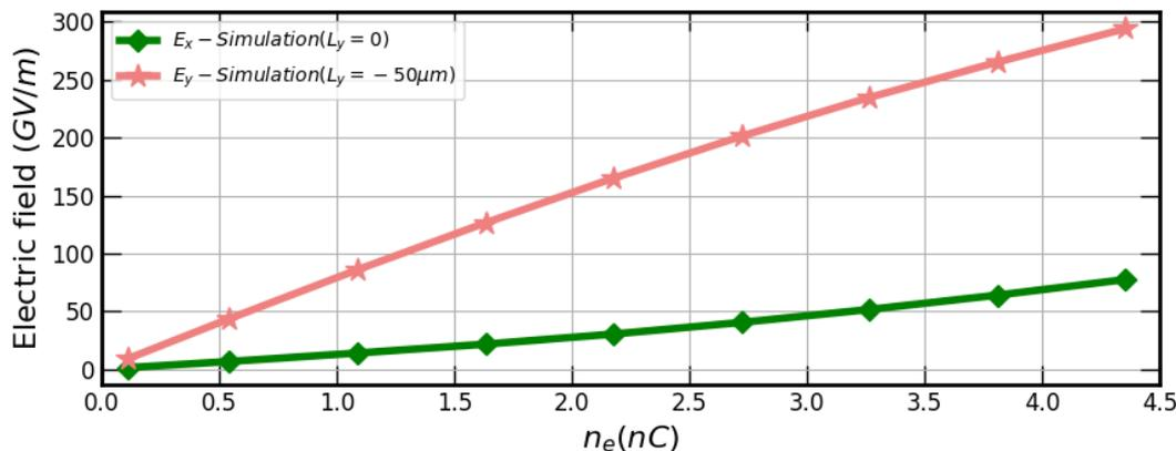
Due to the terahertz radiation from the oscillating electrons continuously, a field of about tens of GV/m, propagates synchronously with the electron beam and accelerates the positron bunch in a stable phase.
