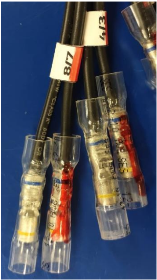
"Samtec" cable splices & 标签
