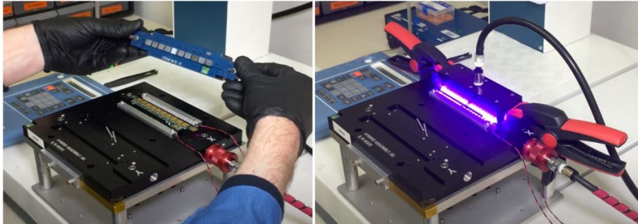
Place ASICS on hybrid flex and UV cure the glue
