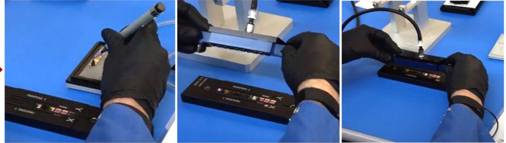
Place ASICs in alignment tray, then pickup with vacuum tool
