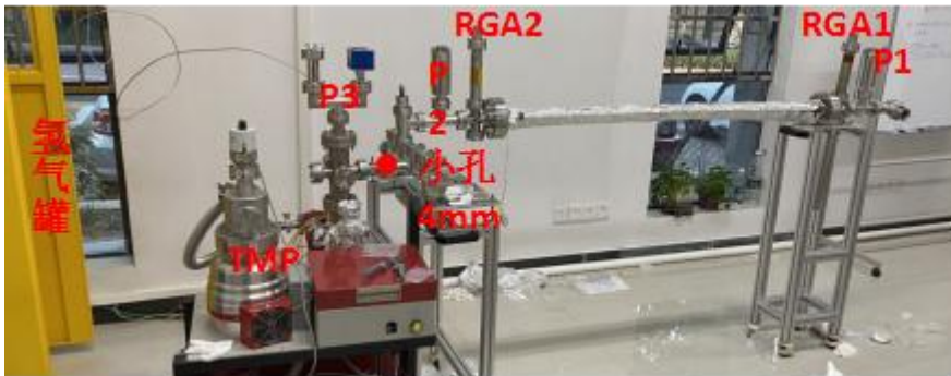
6 m vacuum pipe have been installed on the NEG coating setup
