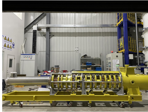
Klystron No. 2 Efficiency 77% (2021)
