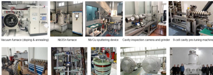
Vacuum furnace (doping & annealing) Nb 3 Sn furnace Nb/Cu sputtering device Cavity inspection camera and grinder 9-cell cavity pre-tuning machine Temperature & X-ray mapping system Second sound cavity quench detection system Helmholtz coil for cavity vertical test Vertical test dewars Horizontal test cryostat
