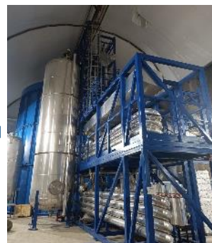
4) Gas stripping to remove Rn and O 2
