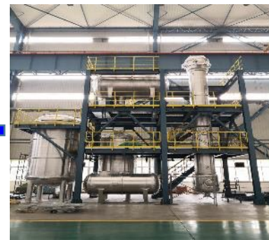
3) Water extraction to remove radioactive impurities
