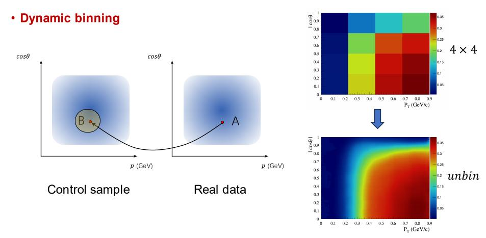
• For a certain point A in the phase space of real data, we can look for its corresponding point B in the control sample, then calculate the efficiency using the neighborhood region of B. The systematic and statistic uncertainty can be balanced by varying the size of neighborhood of B.
