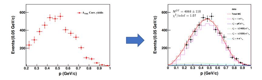
The electron with momentum below 0.2 GeV can not be detected by the spectrometer, the efficiency is extremely low. Extension to the whole region is essential to obtain the total yield.
