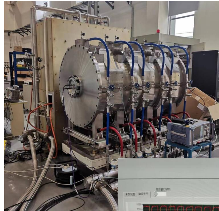
The RF cavity loaded with Magnetic Alloy (MA) for CSNSII
