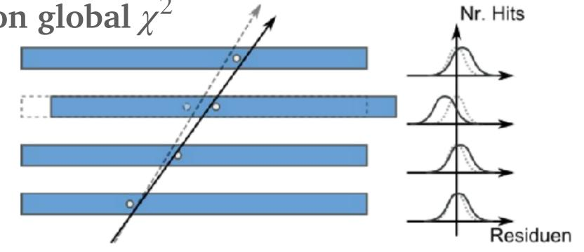
Residual: distance of measured hit with the intersection point of track in the measured chip
