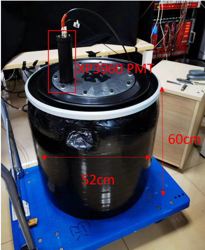
Pure Water tank with Fiber-PMT
