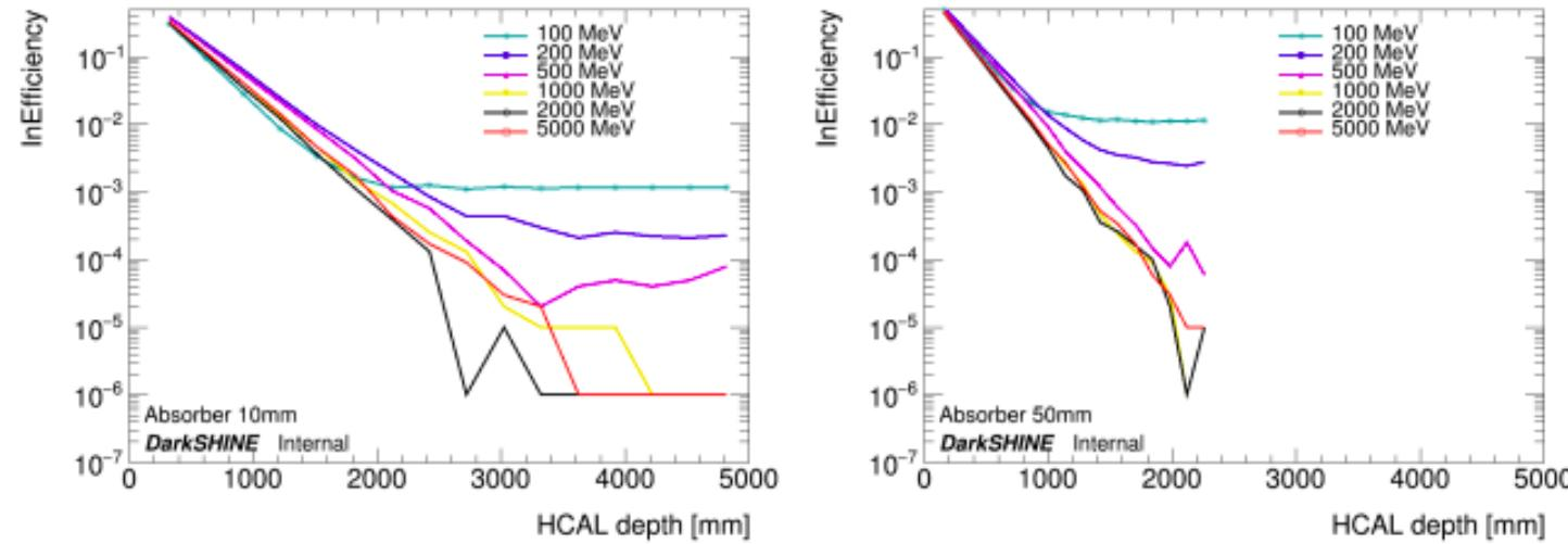
**Figure 7.** Veto inefficiency as a function of detector depth for different beam energy. Different absorber thickness are selected, Left figure is showing effects for 10 mm absorber detectors and right hand side figure is showing effects on 50 mm absorbers.
