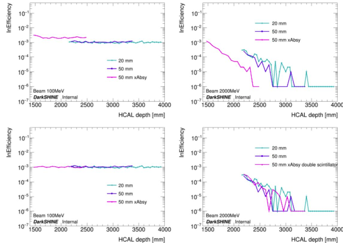
**Figure 8.** Veto inefficiency as a function of detector depth for different absorber thickness and scintillator strategy. 100 and 2000 MeV neutrons are generated to hit towards hadronic calorimeter at its center. Top two plots show the case that scintillator is 1 cm thick, while that in the bottom two plots is 2 cm.
