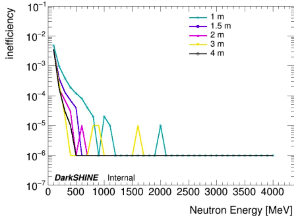
**Figure 5.** Veto inefficiency as a function of different incident neutron energies. Larger size HCAL is showing better veto power as expected due to its capability of acceptance compared with smaller size HCAL designs. To satisfy the weighting limits of the SHINE facility, we decided to use 1.5 m as the final design.
