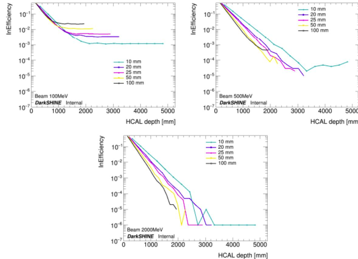
**Figure 6.** Veto inefficiency as a function of detector depth for different absorber thickness. 100,500 and 2000 MeV neutrons are generated to hit towards hadronic calorimeter at its center. Thick absorber thickness would be able to veto neutrons in small depth range.
