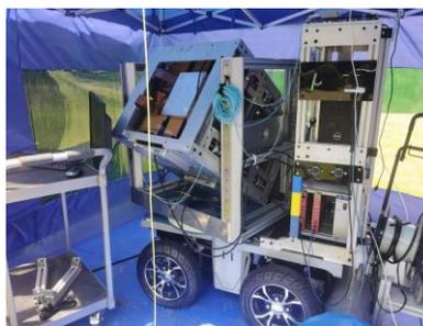
$\mu$ STC:  $\mu$ (muon) Scattering tomography & Transmission imaging facility
