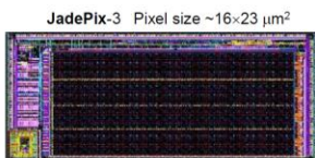
Tower-Jazz 180nm CIS process Resolution 5 microns, 53mW/cm²
