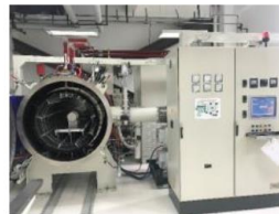
Vacuum furnace (doping & annealing)
