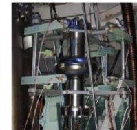
Second sound cavity quench detection system
