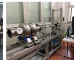
Cavity inspection camera and grinder
