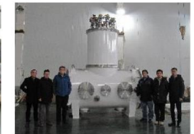
Horizontal test cryostat
