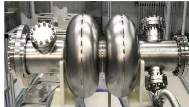
Vertical test of 650 MHz 2-cell cavity
