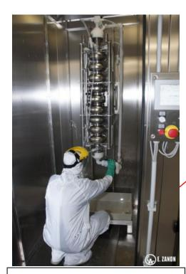
Cabinets for BCP close circuit of the inner / outer cavity surfaces
