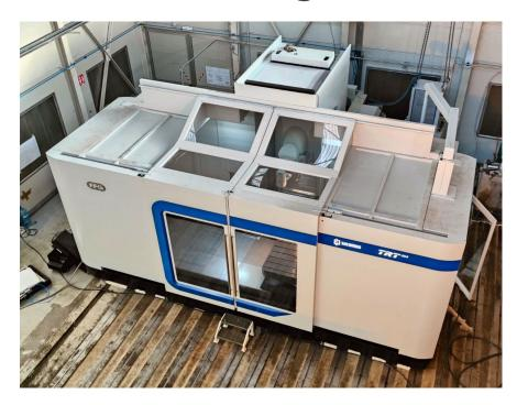
5 axis CNC milling machine 1600x2000x4000 mm
