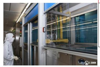
Automatic pluritank station for UT cleaning and rinsing baths water 10 MΩcm and 18 MΩcm
