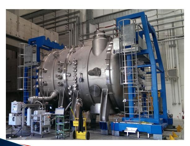
Zanon participated with an international consortium to produce the Ion Source prototype for ITER beam injectors.
