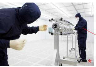
Station for final leak test special equiments for slow-controlled venting of the cavity
