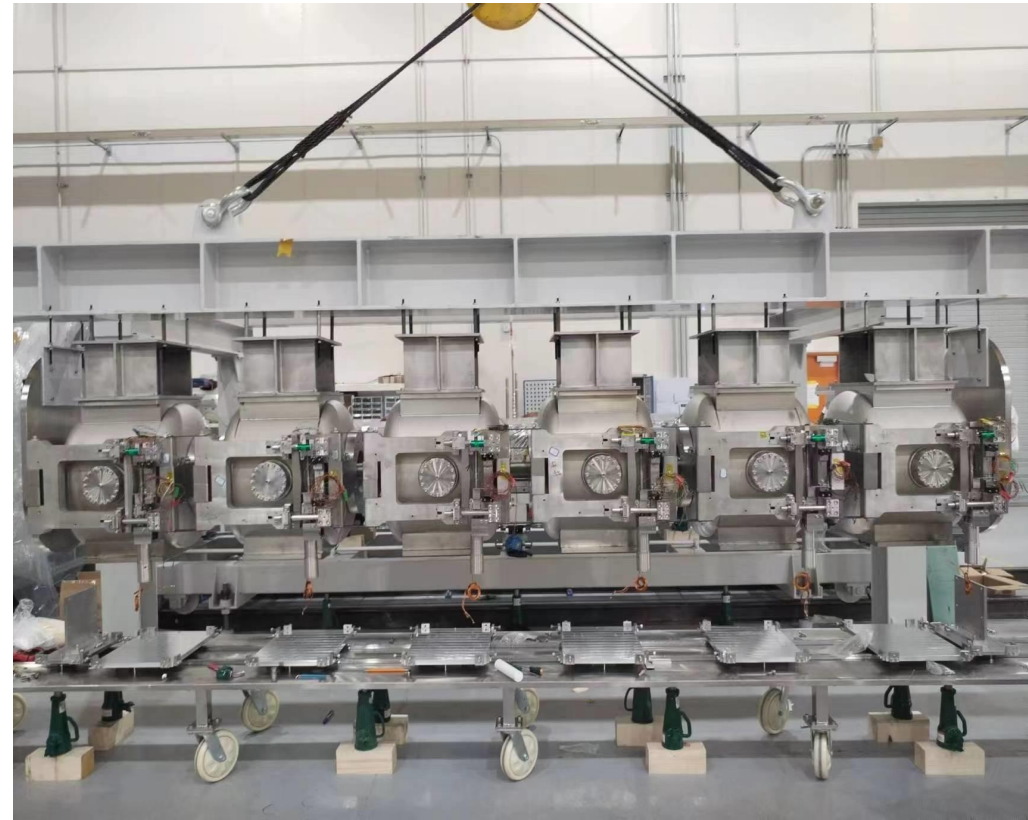
Cavity string on cold mass
