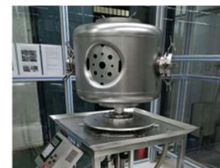
Spoke 051 SSR2超导腔 (325MHz)
