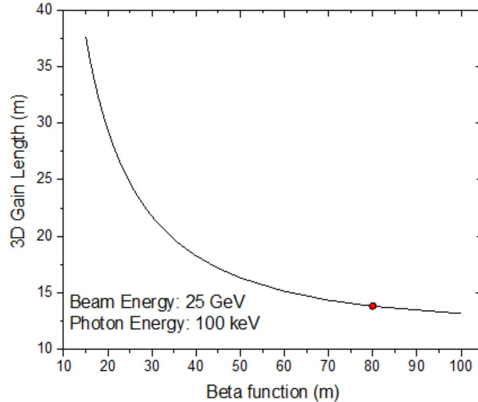
25 GeV beam energy and 80 m beta function is the optimum selection for a reasonable saturation length
