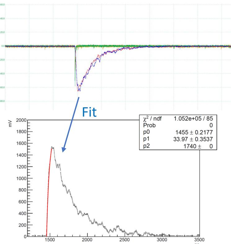
Time Resolution from Waveform Simu
