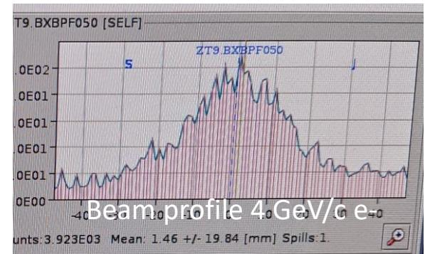
➤ Beam profile: severe changes in the spatial distribution of the beam spot
