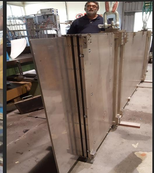
Larger modules (more plates) → bigger machine needed & complicated handling (heavy structure to be moved and rotated several times)
