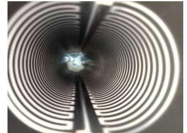
Ceramic chamber with TiN-Ag metallic coating of ladder pattern
