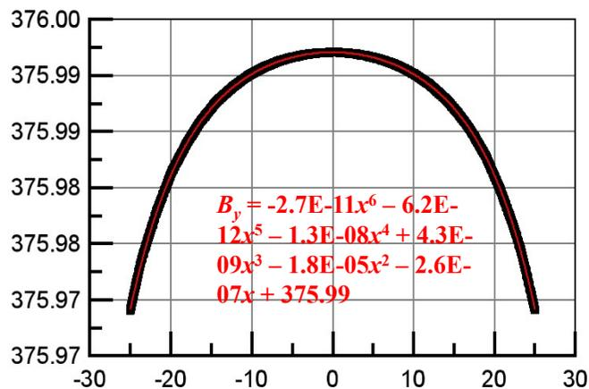
The dipole field is 376Gs, and total field errors is about 0.017 Gs
