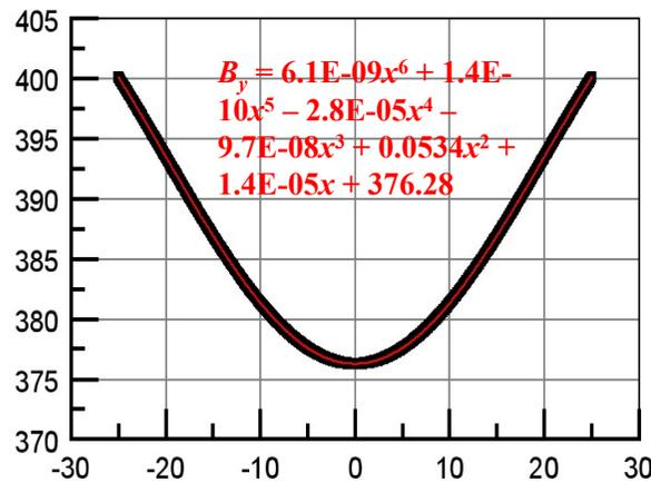
The dipole field is 376Gs and the sextupole field is 10.68T/m<sup>2</sup>
