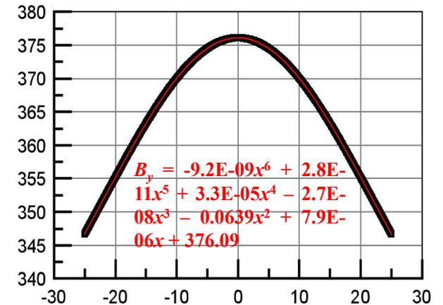
The dipole field is 376Gs and the sextupole field is -12.78T/m<sup>2</sup>
