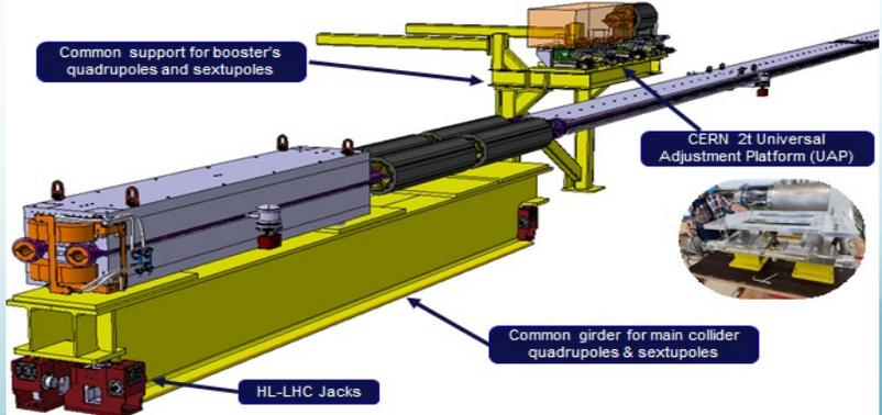
**Vibration mitigation and misalignments control** are crucial to obtain **high luminosity** (CLIC FFS magnet specification displacements 0.2 nm at 4Hz).
