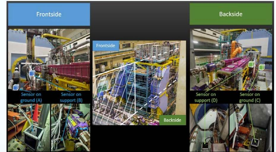
4 seismic sensors (2 each side) BELLE II
