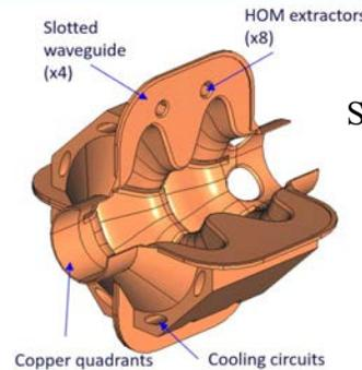
Slotted Waveguide Elliptical cavity (SWELL)
