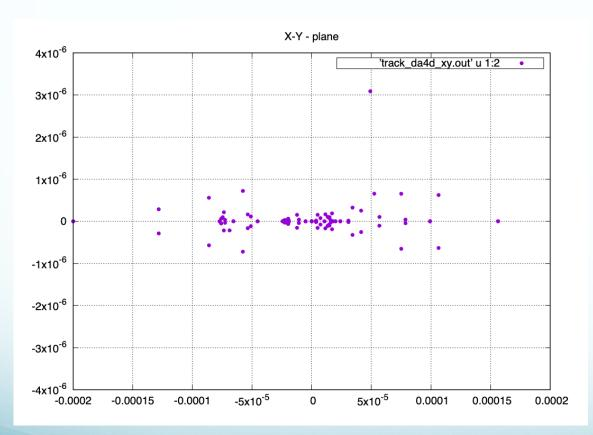
1000 Turns DA Tracking for Monochromatization Mode
