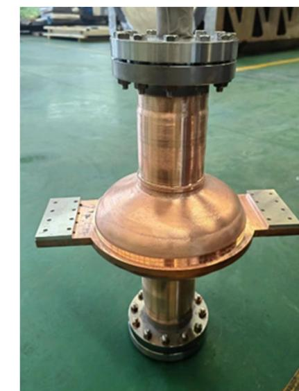
Cold spraying with copper
