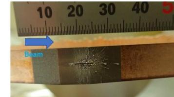
Fig.2 Damage to collimator jaw due to accident beam loss in the SuperKEKB
