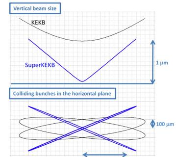
Figure 2: Schematic view of the nanobeam collision scheme.
