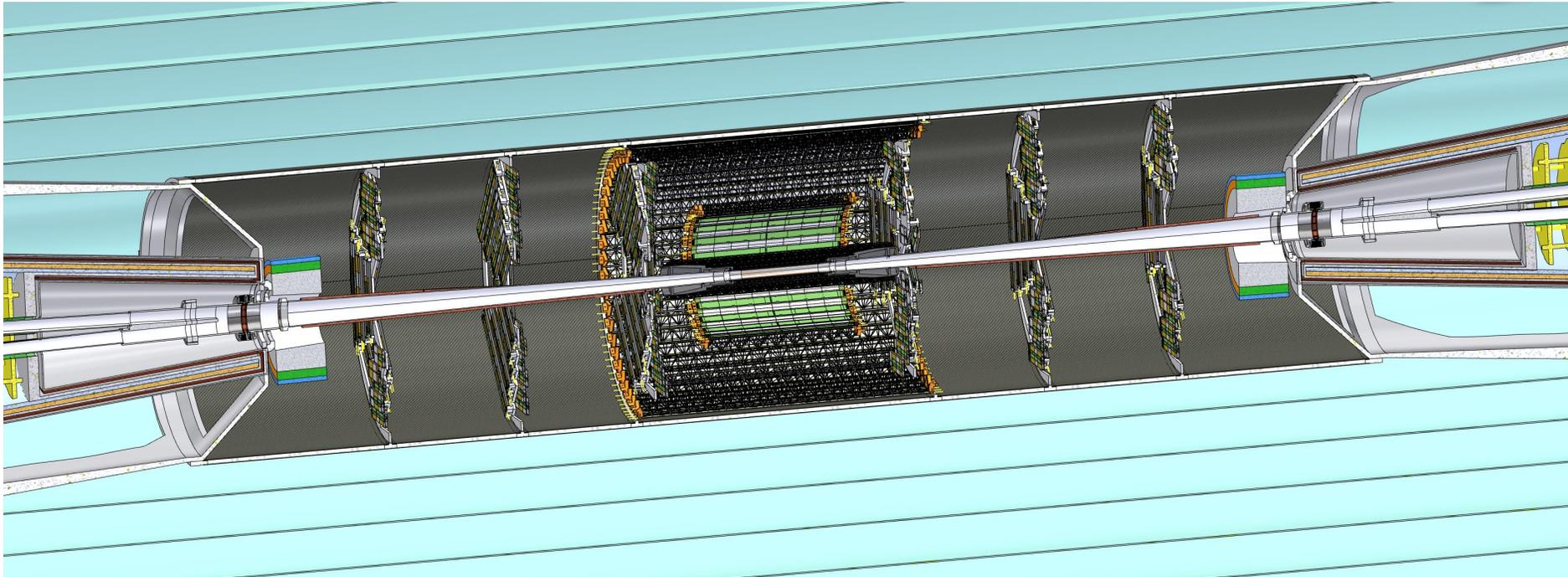
View including the rigid support tube, vertex detector and outer trackers
