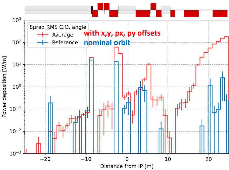
Power deposition from beam core for Z-mode
