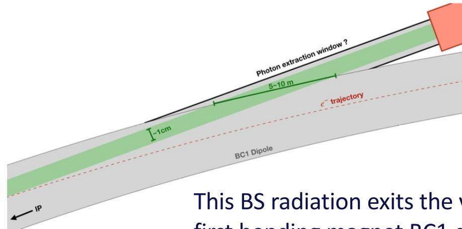
This BS radiation exits the vacuum chamber around the first bending magnet BC1 downstream the IP
