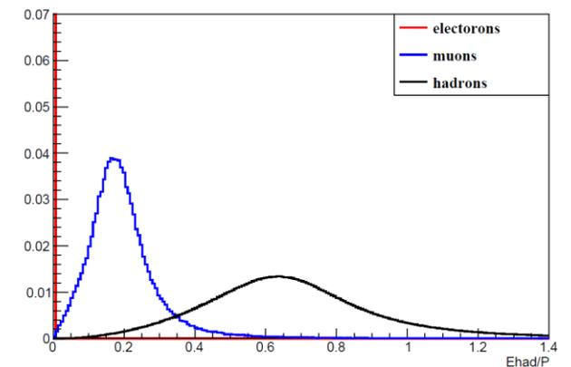
Calorimeters provide energy of photon and neutral particle for jet clustering and lepton/hadron identification
