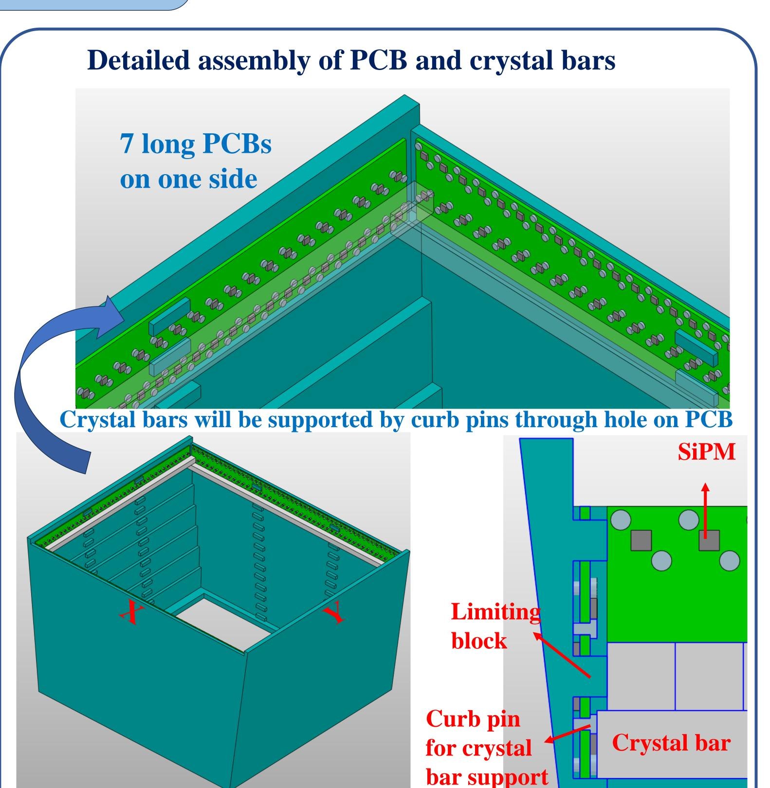
The crystal bars in the X direction are supported by steps every four layers, while the crystal bars in the Y direction are supported by the crystal bars in the X direction; The two ends of the crystal bars are fixed by two curb pins, while the sides are fixed by two limiting blocks.
