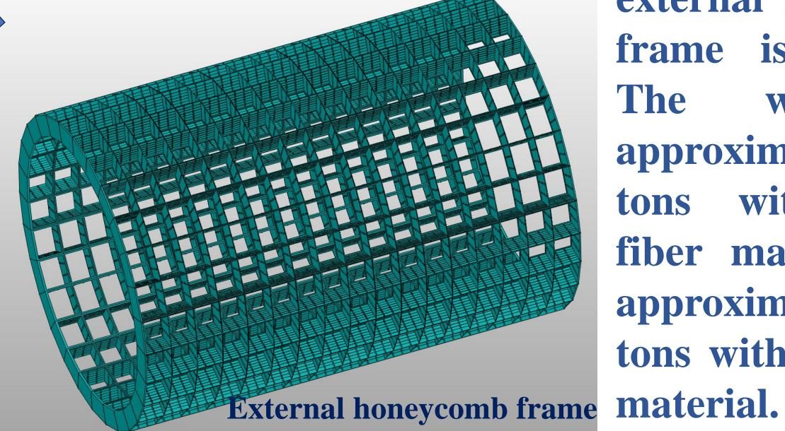
The length of the external honeycomb frame is 6660mm, The weight approximately tons with carbon fiber material, and approximately tons with aluminum
