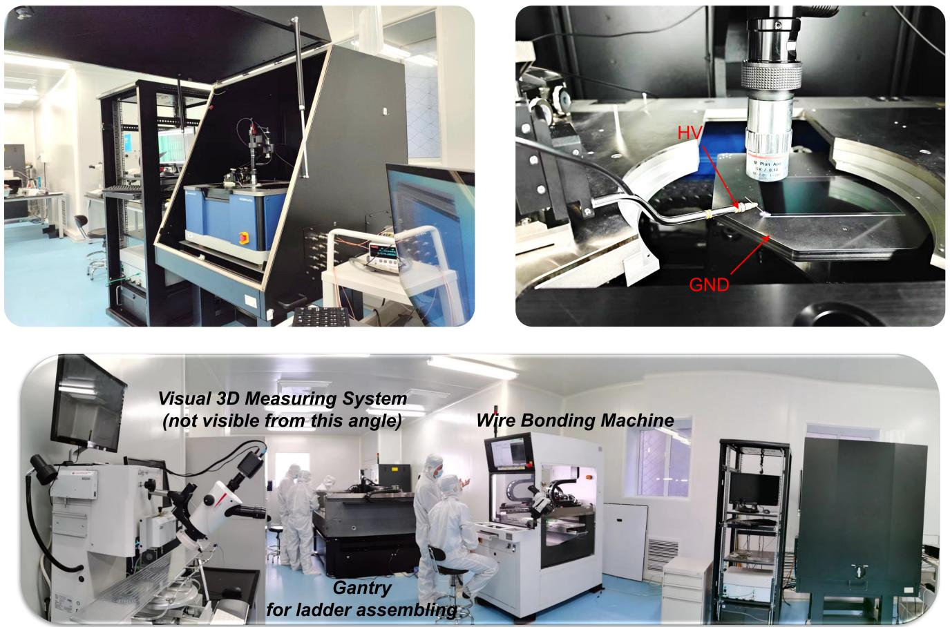
Once the ladder is assembled, alignment precision is assessed using an optical metrology system. The coordinates of all four fiducial marks on the SSDs are measured, and these measurements determine the alignment. We fit the X and Y coordinates to assess deviations along the vertical axis, as well as the vertical distances between two SSDs. The optimal vertical gap between two SSDs should be around 150µm. Thus far, we have achieved our goal of  $5\mu m$  precision along the horizontal axis.
