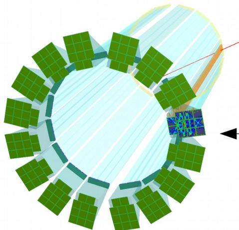
Accumulated hit pattern from 1000 K<sup>+</sup> at 3.5 GeV/c and 25° polar angle
