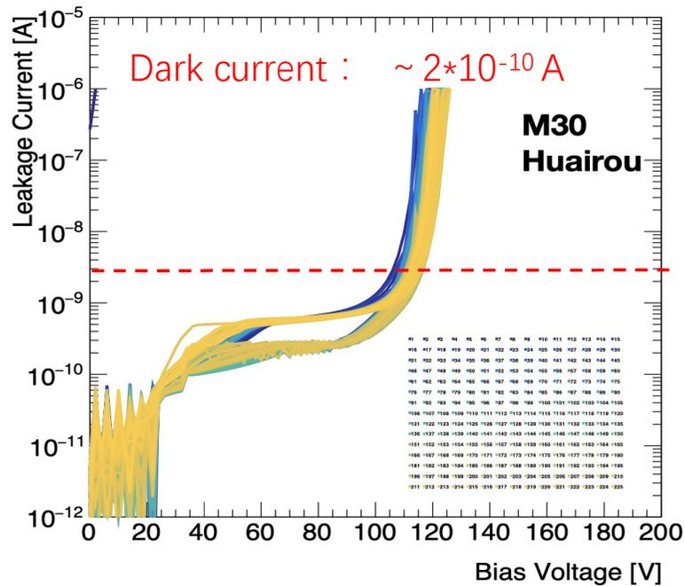
Leakage current of LGAD after irradiation
