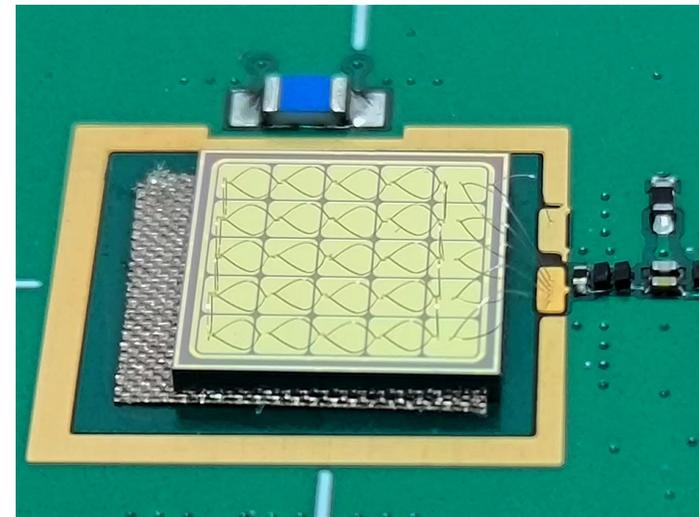
5\*5 Large area LGAD sensor Connected by wire bonding
