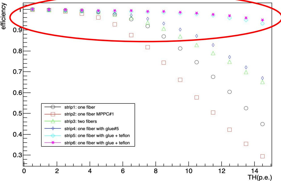
The strips with optical glue and Teflon have highest efficiency, **keeping upon 98% at threshold of 10 p.e.**
