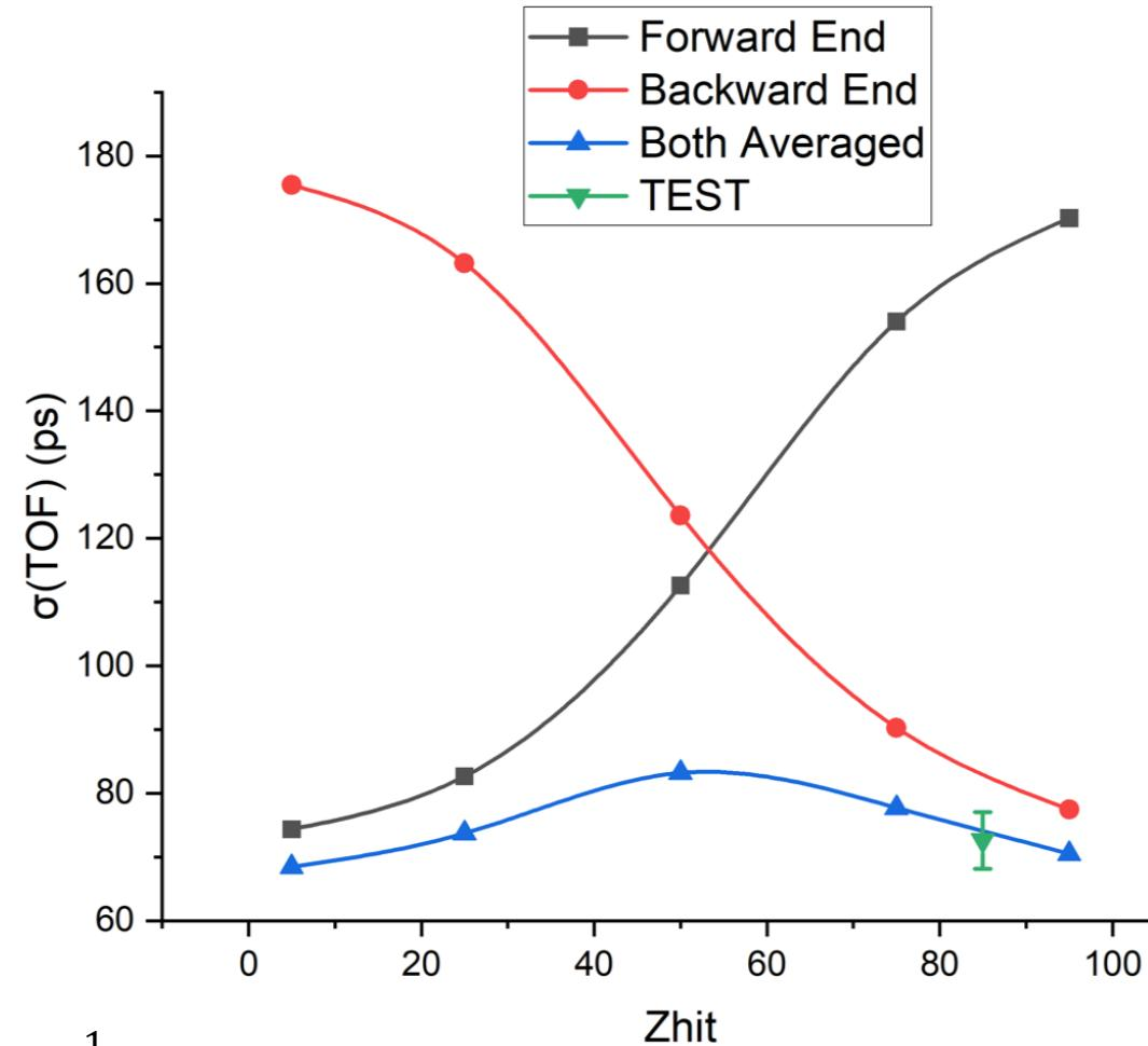
—▲— Both Averaged Calculated by the error transfer formula  $\frac{1}{\sigma_{s.c.}^2} = \frac{1}{\sigma_F^2} + \frac{1}{\sigma_B^2}$ .
