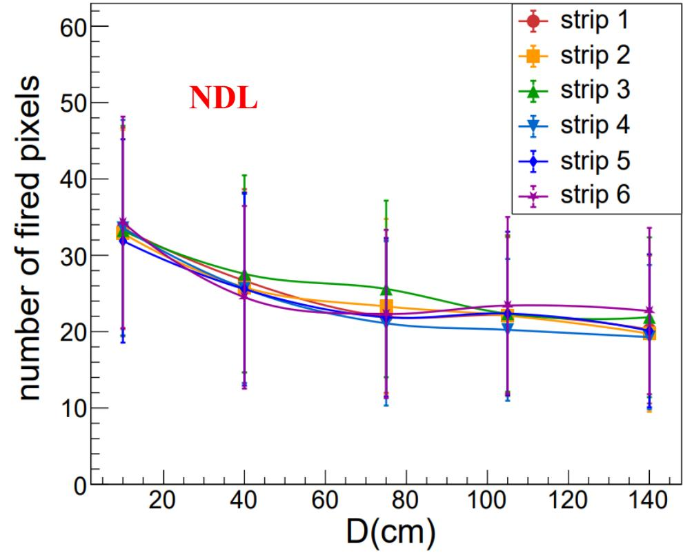
Wavelength-shifting fiber keeps good photon collection at long distance
