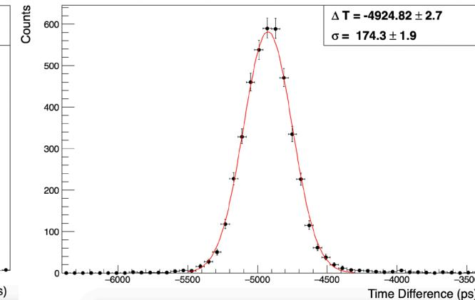
Spatial resolution according to  $\Delta T$  between 3 and 4 should be  $\sim 0.17 \times \frac{30}{n} \text{ cm}$ , which is 3.4cm
