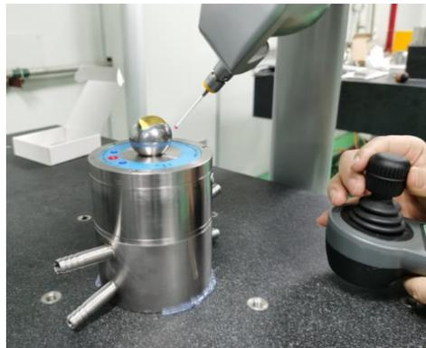
Figure 4 Calibration of the bowl's size using the three-coordinate measuring machine (CMM)
