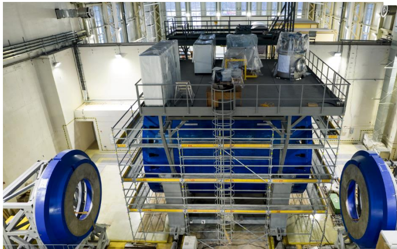
The magnet consists of Solenoid inside Iron Token and two correction coils inside of Endcaps
