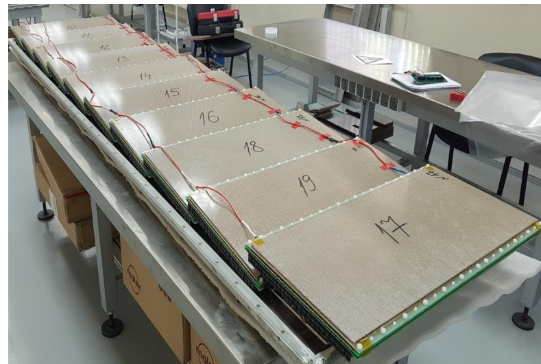
TOF modules assembling
