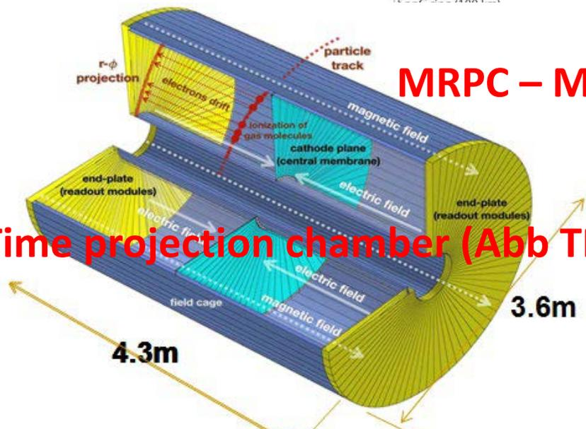
Particle Identification (PID) System
