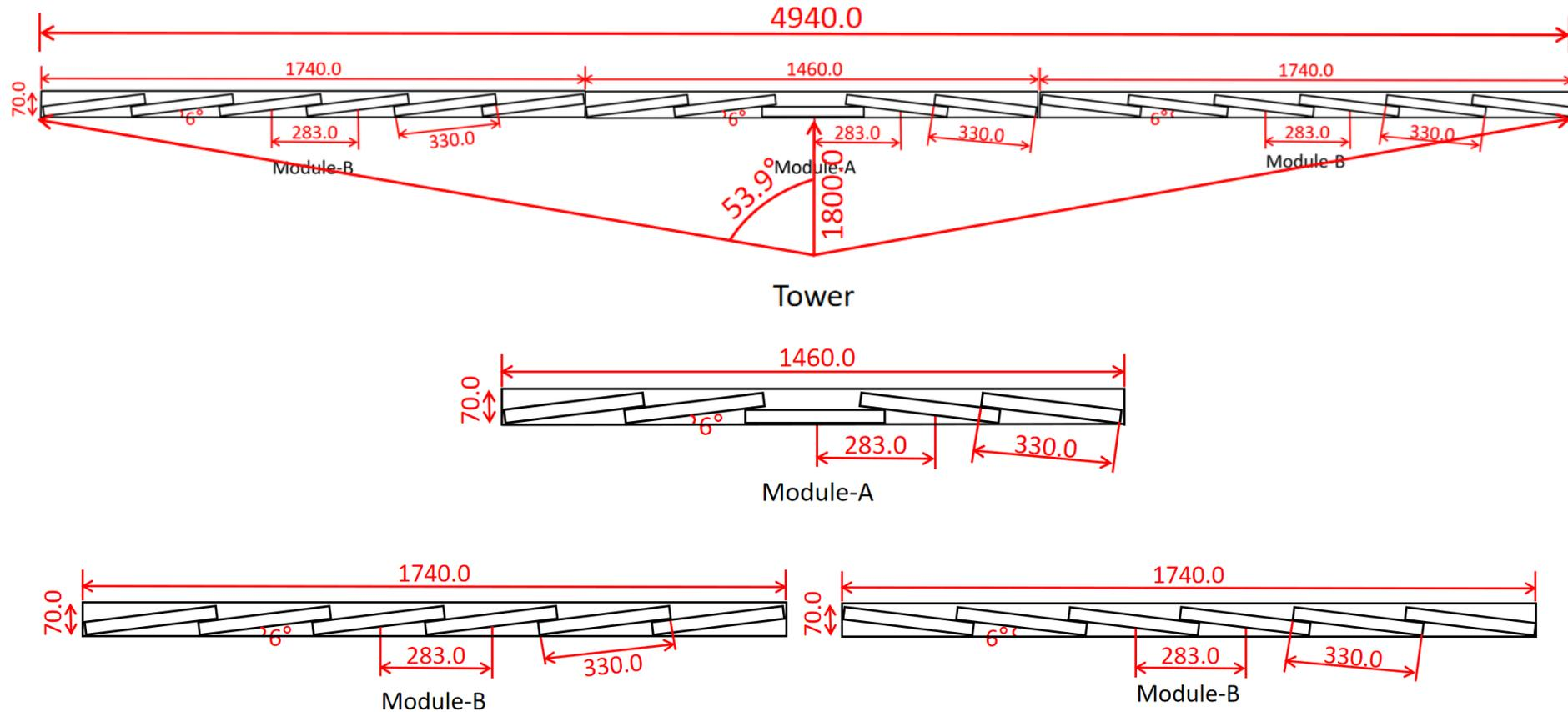
Arrangement of MRPCs inside the box along the beam direction
