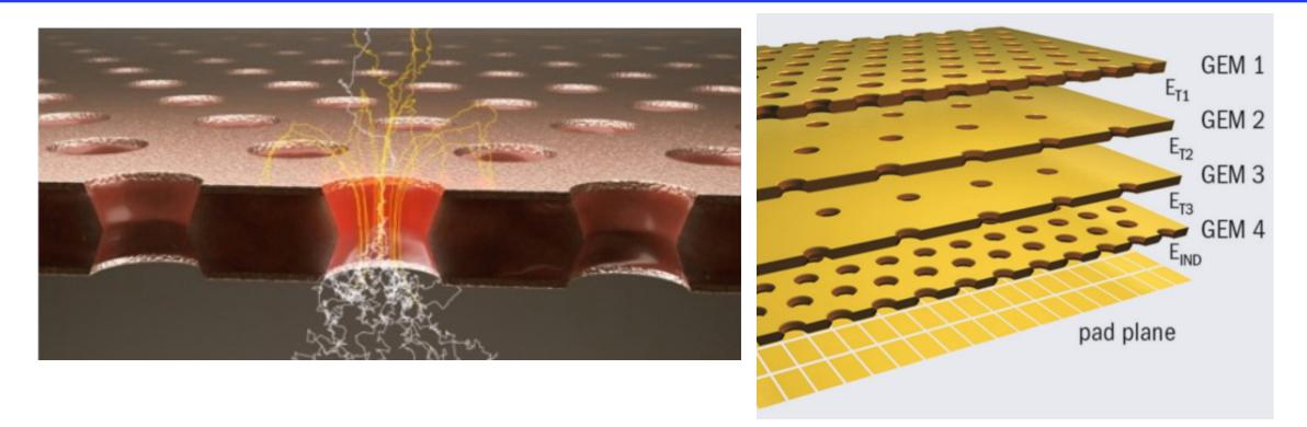
Upgrade front end electronics by Gaseous Electron Multiplier (GEM) foils
