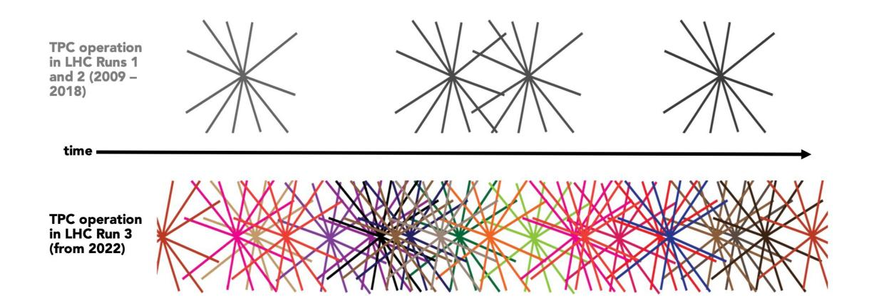
From triggered readout (Run 1&2) to continuous readout with GEMs (Run3)
