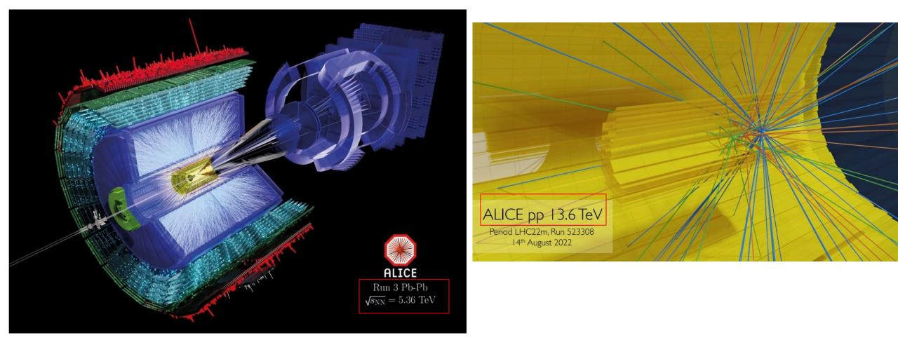
The updated TPC with GEM readout allows to take the data at the IR at 50KHz for Pb-Pb at 5.35 TeV and 500k for pp at 13.6 TeV collisions
