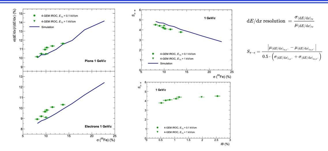
Extensive studies demonstrated that the dE/dx resolution slightly worsens with increasing occupancy from 5.5% in isolated pp events without pileup to about 7.5% in central Pb–Pb at 50 kHz
