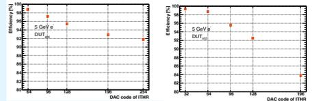
The detection efficiency also can reach 99% for the vertex detector prototype at the lowest setting threshold
