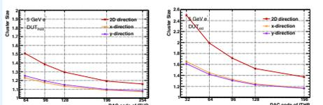
The DUT with the standard process shows more charge-sharing effects
