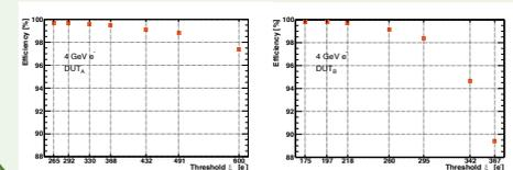
The detection efficiency for both process can reach 99% at the lowest threshold
